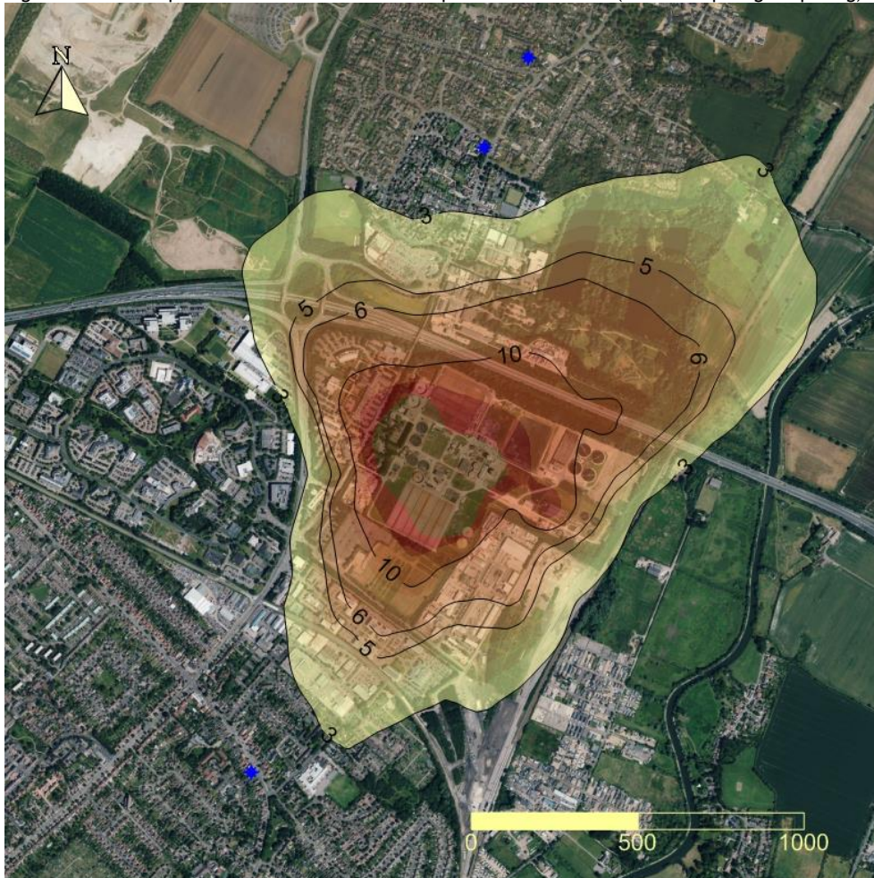
Figure 9: Current operational conditions model output - 2015 Met data (100m receptor grid spacing)
